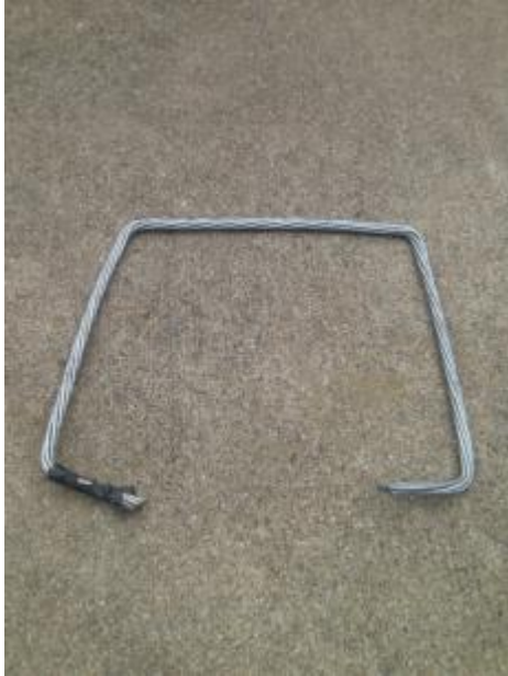
Figure 1.6: Guy wire formed to be placed in wet concrete of anchors to create an anchor handle.
