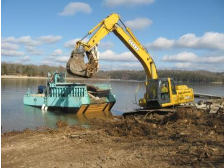
Figure 1.4: 200-class, 45,000 pound excavator loading stumps onto the rock barge.
