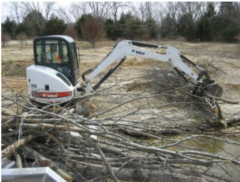
Figure 1.3: 50-class, 10,000 pound excavator handling trees to load onto the Table Rock Lake habitat barge.
